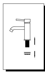
2. Screw the Hot and Cold supply hoses (18) to the copper waterways/ inlets (9).
