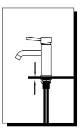
5. Once in place, proceed to attach gasket (13) and finally, re-attach the lock nut. Be sure to tighten lock nut into place so faucet stands securelly on its own.
